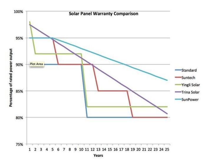
The majority of manufacturers offer the 25-year standard solar panel warranty, which means that power output should not be less than 80% of rated power after 25 years.
